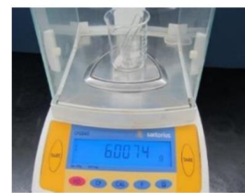
Electronic Balance (resolution 0.01 g)
