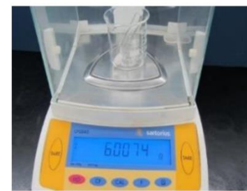
Electronic Balance (resolution 0.01 g)
