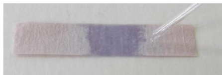
Figure T15-1 Using litmus paper to test acid base property
