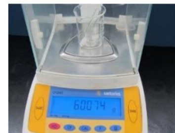
Electronic Balance (resolution 0.01 g)
