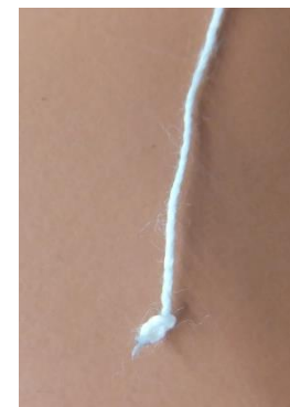
Solution concentration too low; or solution had not been cooled down to RT
