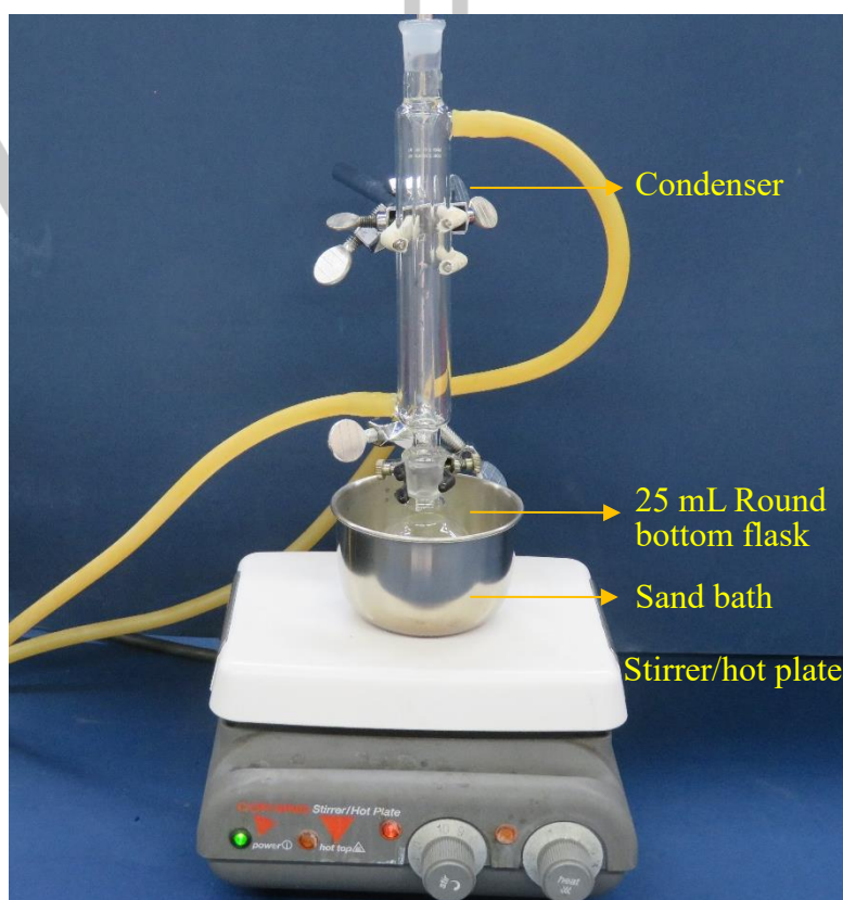
Figure 16-3 Reflux system for synthesis of gold nanoparticles
