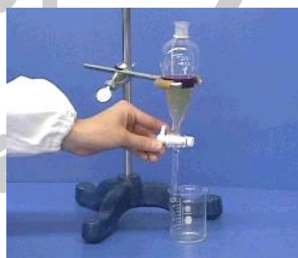
Figure 19-3 Support the funnel using an iron ring
